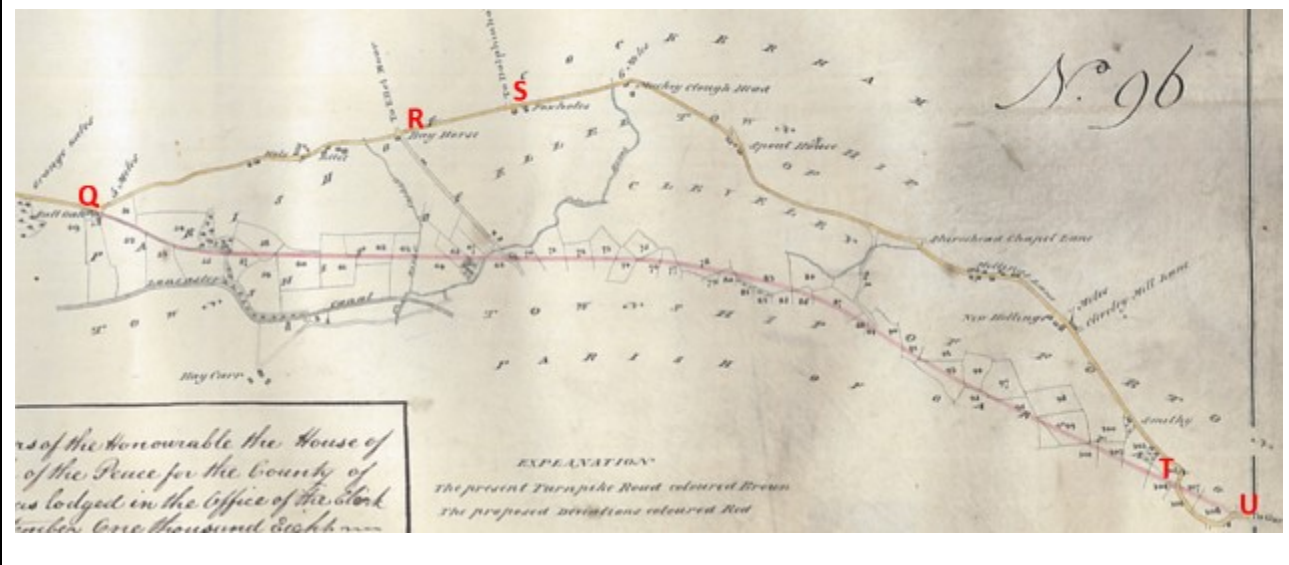
Proposed deviation of toll road in Galgate with modern OS map showing new route constructed and the retention of old toll road as a public vehicular route
